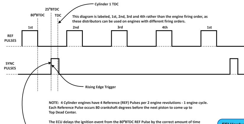
to deliver the ignition spark at the correct crankshaft angle for any given engine condition
