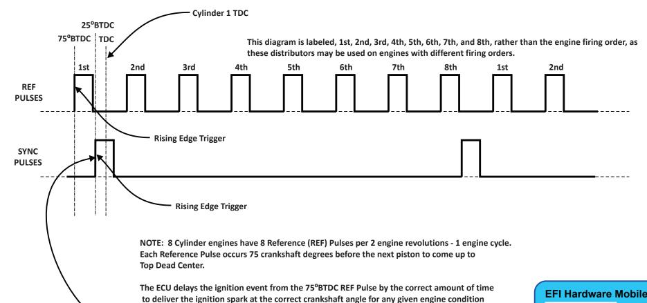
The SYNC Pulse tells the ECU when the engine returns back to the first cylinder in the firing order.
