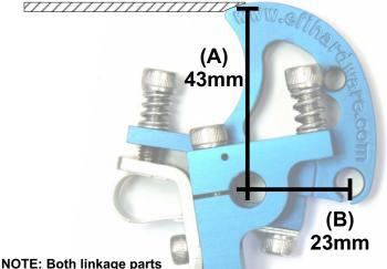
must be fitted to a round 8mm or 5/16" throttle shaft. Do not mount the linkage to a "D"sectioned shaft, as the Throttle Stop will come loose and move on the shaft.
