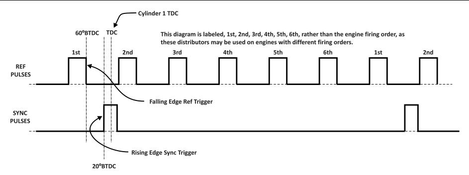
NOTE: 6 Cylinder engines have 6 Reference (REF) Pulses per 2 engine revolutions - 1 engine cycle. Each Reference Pulse occurs 60 crankshaft degrees before the next piston to come up to its **Top Dead Center.**
