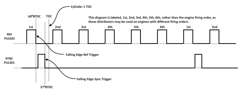
NOTE: 6 Cylinder engines have 6 Reference (REF) Pulses per 2 engine revolutions - 1 engine cycle. Each Reference Pulse occurs 60 crankshaft degrees before the next piston to come up to **Top Dead Center.**
