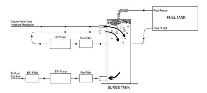
Every item in the fuel system from the Fuel Tank to the Fuel Injectors must be sized correctly to suit the expected engine power, and the type of fuel you are running your engine on.
