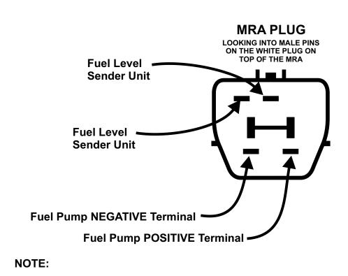
The Fuel Level Sender is a simple variable resistor. The wiring does not have specific Positive or Negative Terminals. Hence, you can wire it either way around. MRA ELECTRICAL SPECIFICATIONS:
