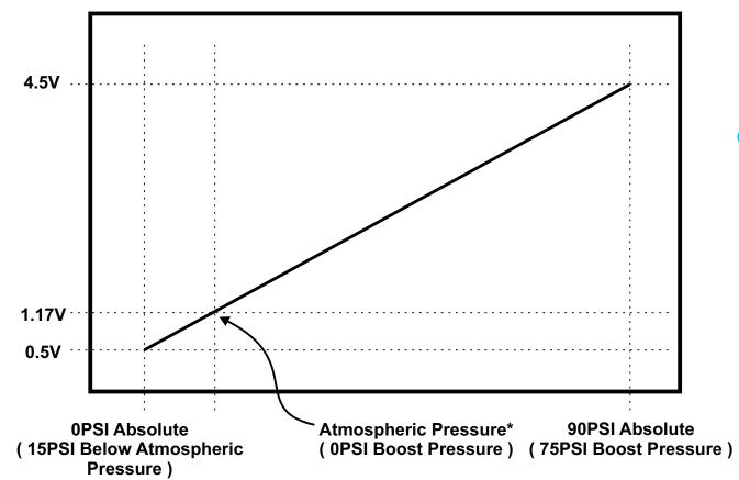
\*NOTE: This is an estimate of the voltage as Atmospheric Pressure changes with altitude and weather conditions
