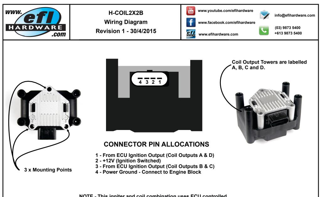
NOTE - This igniter and coil combination uses ECU controlled dwell time. It includes 2 igniter channels and 2 dual ended coils. Great for 4 cylinder applications (use 2 for 8 cylinder applications).
