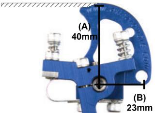
NOTE: Both linkage parts must be fitted to a round 8mm or 5/16" throttle shaft. Do not mount the linkage to a "D"sectioned shaft, as the Throttle Stop will come loose and move on the shaft.
